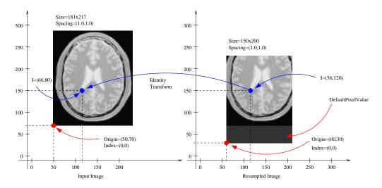
Figure 6.46: Effect of selecting the origin of the input image with ResampleImageFilter.
