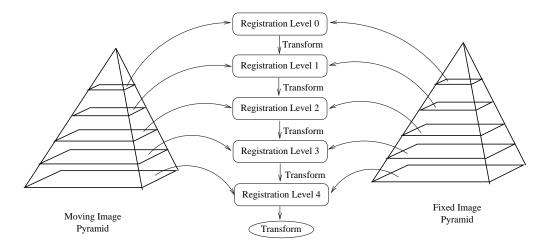
Figure 8.37: Conceptual representation of the multi-resolution registration process.
