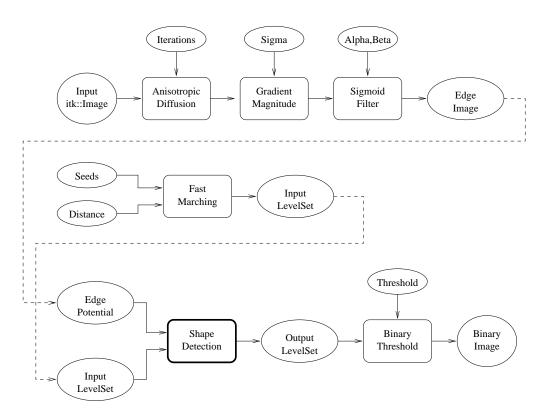
$Figure~9.18: \ Collaboration~diagram~for~the~Shape Detection Level SetImage Filter~applied~to~a~segmentation~task.$
