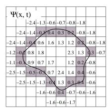
Figure 9.14: The implicit level set surface  $\Gamma$  is the black line superimposed over the image grid. The location of the surface is interpolated by the image pixel values. The grid pixels closest to the implicit surface are shown in gray.
