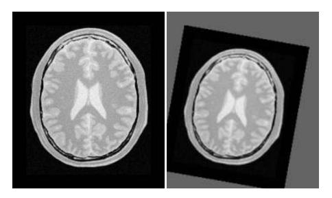
Figure 6.54: Effect of the resample filter rotating and scaling an image.
