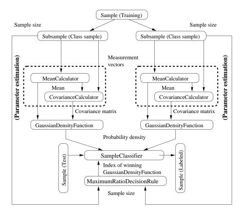
$Figure\ 10.7\hbox{: Bayesian plug-in classifier for two Gaussian classes.}$
