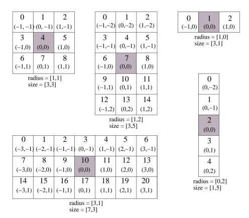
Figure 11.6: Several possible 2D neighborhood iterator shapes are shown along with their radii and sizes. A neighborhood pixel can be dereferenced by its integer index (top) or its offset from the center (bottom). The center pixel of each iterator is shaded.
