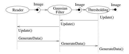
Figure 13.3: Sequence of the Data Pipeline updating mechanism
