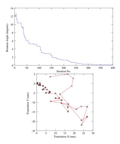
Figure 8.61: Plots of the angle and translation parameters for a registration process between an spatial object and an image.
