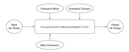
Figure 9.37: Inputs and outputs to FuzzyConnectednessImageFilter segmentation algorithm.
