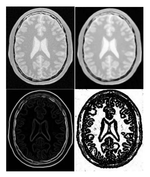
Figure 9.19: Images generated by the segmentation process based on the ShapeDetectionLevelSetImageFilter. From left to right and top to bottom: input image to be segmented, image smoothed with an edge-preserving smoothing filter, gradient magnitude of the smoothed image, sigmoid of the gradient magnitude. This last image, the sigmoid, is used to compute the speed term for the front propagation.
