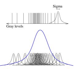
Figure 8.47: In Parzen windowing, a continuous density function is constructed by superimposing kernel functions (Gaussian function in this case) centered on the intensity samples obtained from the image.
