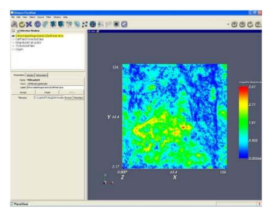
Figure 8.53: Deformation field magnitudes displayed using Paraview
