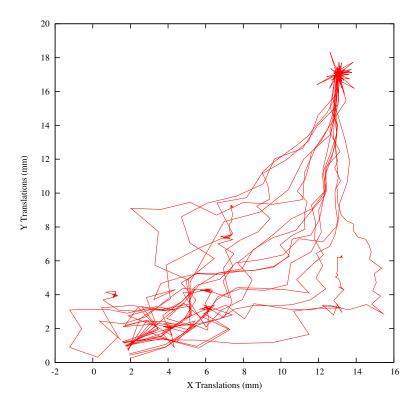
Figure 8.15: Sensitivity of the optimization path to the number of Bins used for estimating the value of Mutual Information with Mattes et al. approach.
