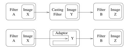
Figure 12.1: The difference between using a CastImageFilter and an ImageAdaptor. ImageAdaptors convert pixel values when they are accessed by iterators. Thus, they do not produces an intermediate image. In the example illustrated by this figure, the *Image* Y is not created by the ImageAdaptor; instead, the image is simulated on the fly each time an iterator from the filter downstream attempts to access the image data.
