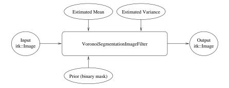
Figure 9.40: Input and output to the VoronoiSegmentationImageFilter.
