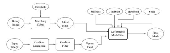
Figure 9.45: Collaboration diagram for the DeformableMesh3DFilter applied to a segmentation task.
