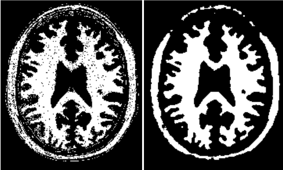
Figure 2.16: Effect of the BinaryMedianImageFilter on a slice from a MRI proton density brain image that has been thresholded in order to produce a binary image.
