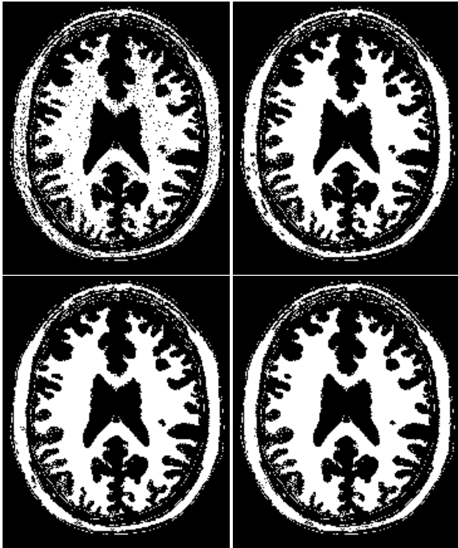
Figure 6.19: Effect of the VotingBinaryHoleFillingImageFilter on a slice from a MRI proton density brain image that has been thresholded in order to produce a binary image. The output images have used radius 1, 2 and 3 respectively.
